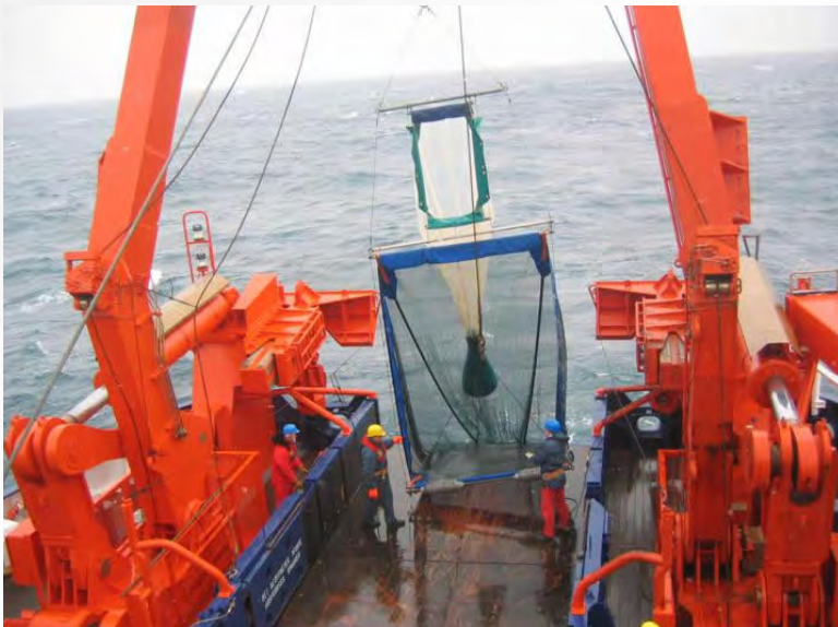
Photograph of the stern part with trawl systems to collect data from the plankton (CSIC source)
