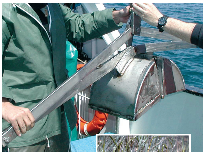
ABOVE: Sampling the sediment. A van Veen drag is a common technique used to get the samples.
